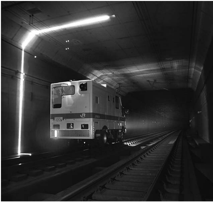
Tunnel Lining Scanning Car (TuLIS)
