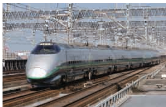
Series 400 with smaller loading gauge for through services between Tokyo and Yamagata via Fukushima (JR East)
