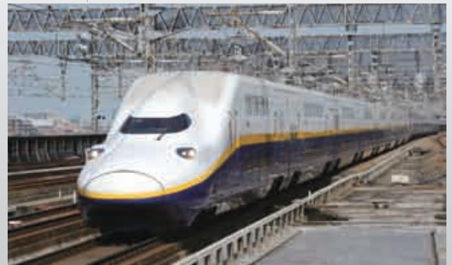
The Series E4 Max distinctive nose shape improves aerodynamic performance at high speeds. (JR East)
