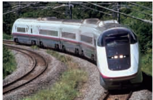
Series E3 with smaller loading gauge for through services between Tokyo and Akita via Morioka (JR East)
