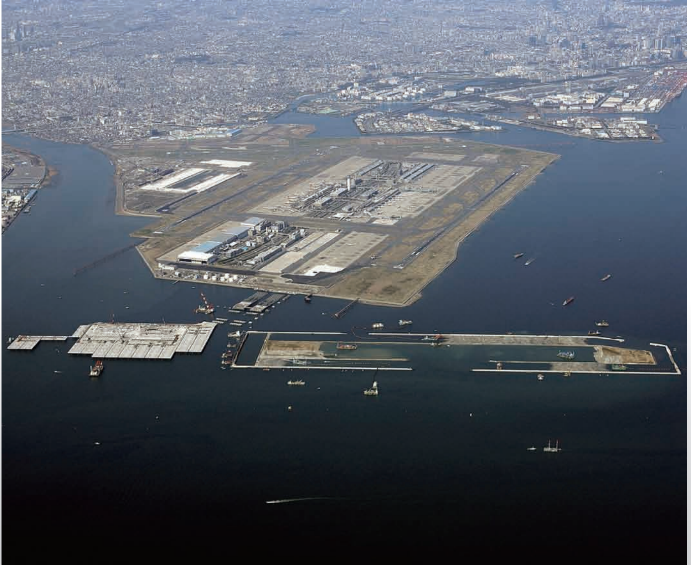
Aerial view of Haneda's construction site; the long rectangle in the foreground will be runway D to be opened in October 2010 (Tokyo International Airport Office)
