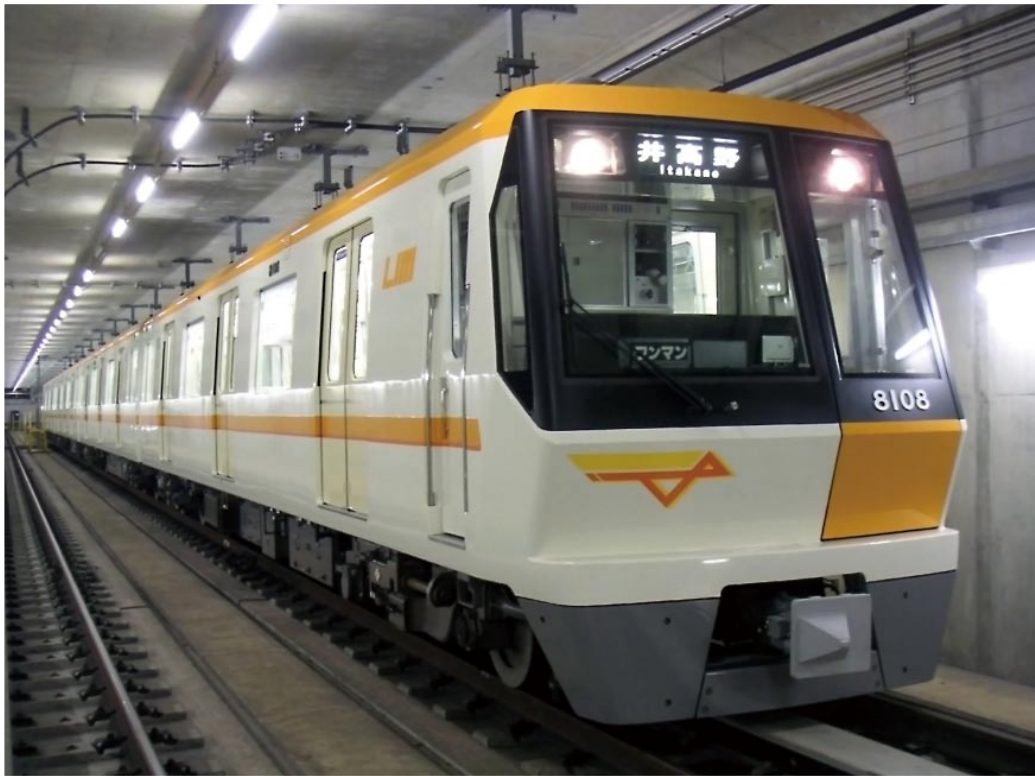
Four-car train set (15 m/car) using same rolling stock as Nagahori Tsurumi-ryokuchi Line (Japan Subway Association)
