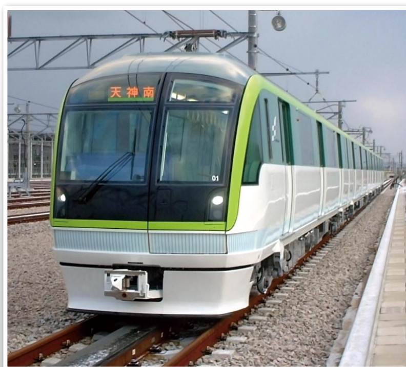
Four-car train set (16 m/car) waiting to depart aboveground depot (Japan Subway Association)
