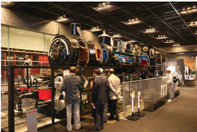
Cutaway of 9850 Class steam locomotive showing internal structure
