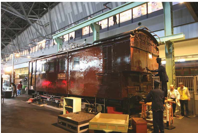
Observing inspection and repair of ED40 train
