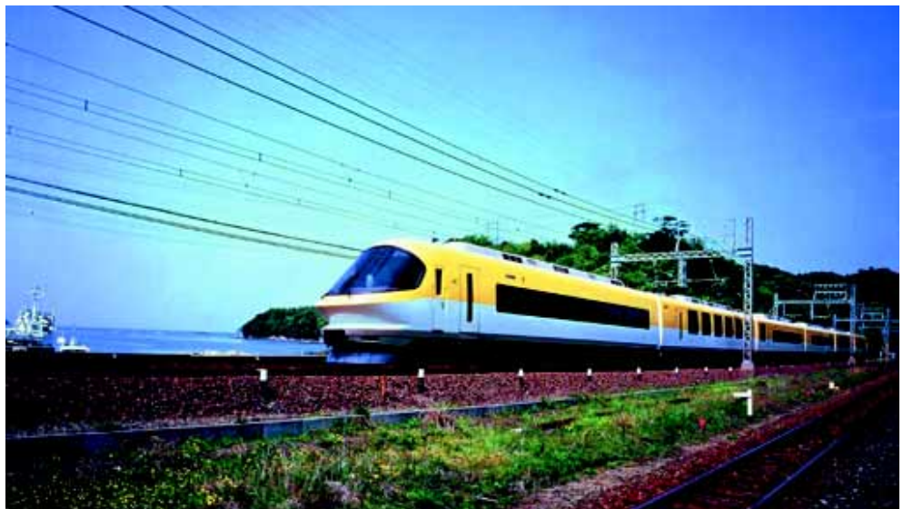
Kintetsu's Series 23000 Ise-Shima Liner limited-express train (1994). Co-designed by Mr Kimura, industrial designer Mr Masamichi Tezeni (1935– 2005), Professor Emeritus Rikuhei Yamauchi of Kyoto Institute of Technology and Kinki Sharyo. (Kintetsu)
