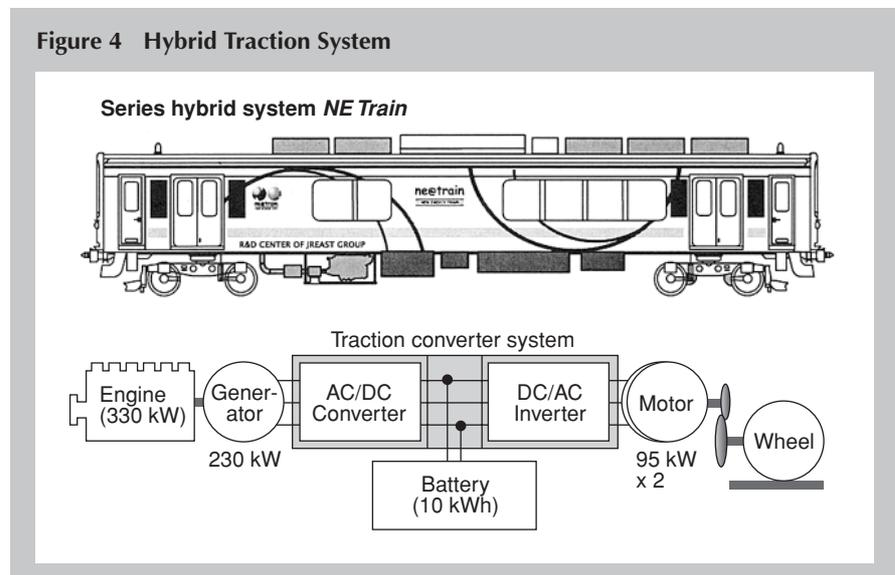
conventional diesel-powered trains, making it possible to increase energy savings via regenerated power. The system uses a series-hybrid configuration designed to allow immediate system conversion (by replacing the engine generator with a fuel-cell unit) in the future
