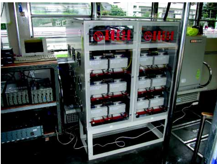
RTRI's battery-powered tramcar eliminating overhead wires (top) and its on-board battery unit (bottom) with measuring equipment on left and battery equipment on right
