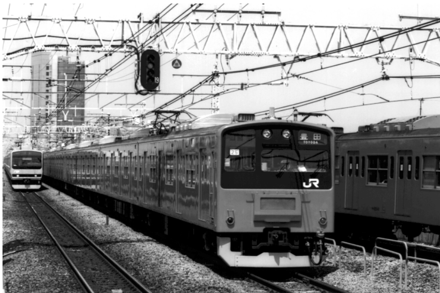
JR East's Series 201 rapid train (right) and Series 209 local train (left) running parallel to each other on quadruple track between Mitaka and Ochanomizu on Chuo Line (Author)
