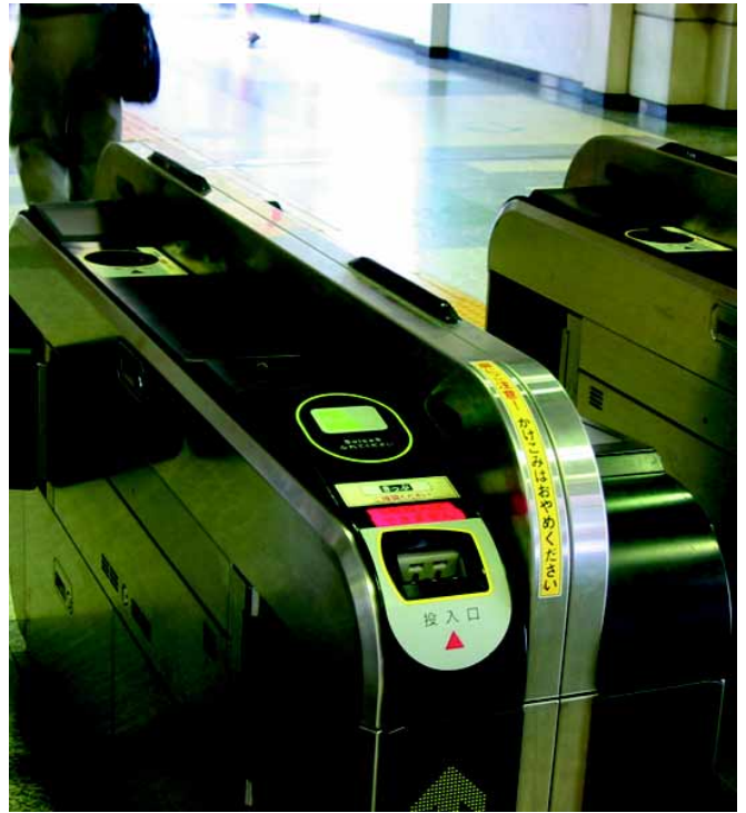
Current automatic gate has both a slot for conventional magnetic cards and a touch-and-go reader/writer for Suica.
