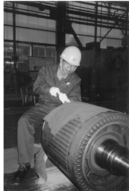
Servicing commutator at Tsuchizaki Workshop in Akita (EJRCF)
