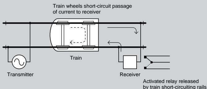
Figure 2 Automatic Block Signalling System
