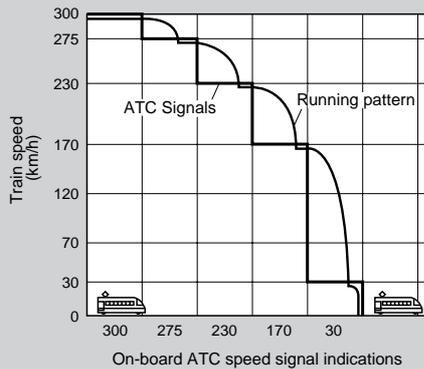
**Figure 6 Digital ATC Train Running Pattern**
