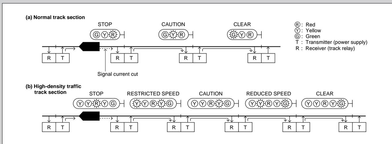
Figure 3 Operation of ATS-S System
