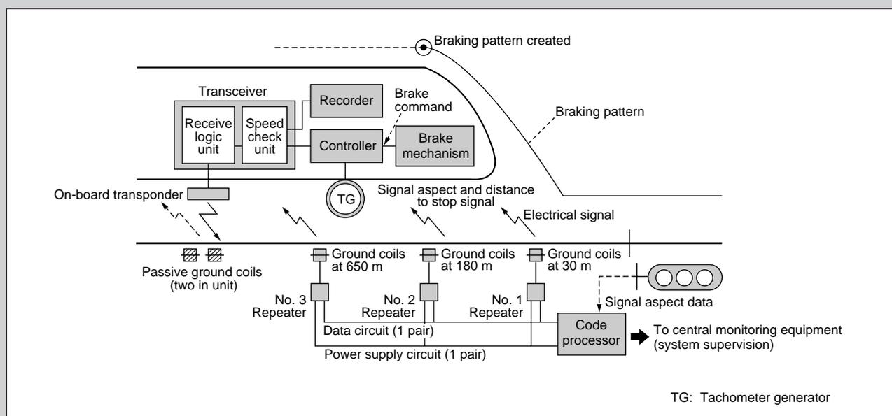
**Figure 5 ATC Train Running Pattern**
