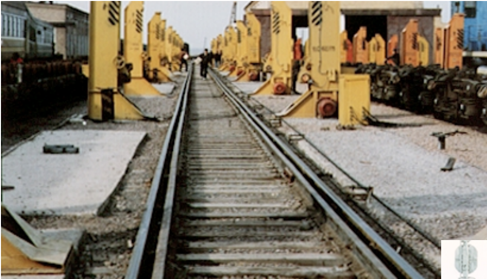
A bogie-changing track at Druzhba Station, Kazakhstan. Bogies are removed and replaced while coaches are lifted by hydraulic jacks.
