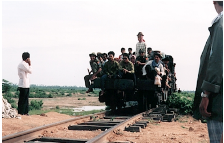
An open freight wagon coupled as a mine-sweeper in front of a valuable locomotive provides a good (but dangerous) view.
